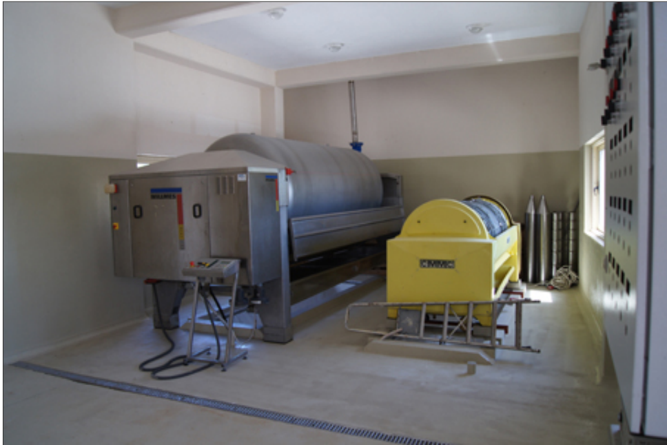
The two horizontal grape presses; Pneumatic on the left and its ancestor on the right.
